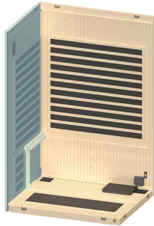
Figure 5. Installing Left Wall Section
