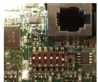
Figure 4 DIP switch positions for using a heater
