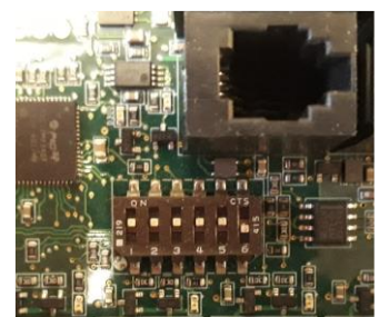
Figure 6 DIP switch positions for using a heater
