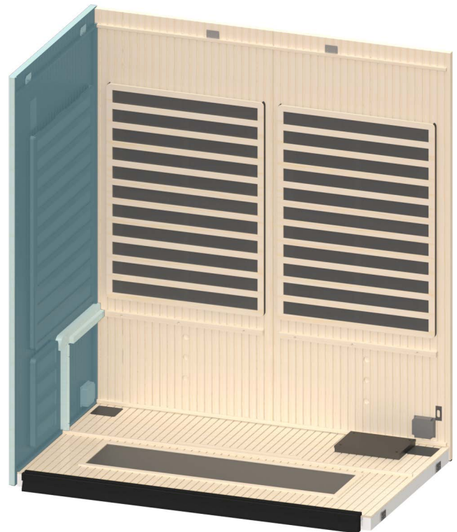
Figure 6. Installing Left Wall Section
