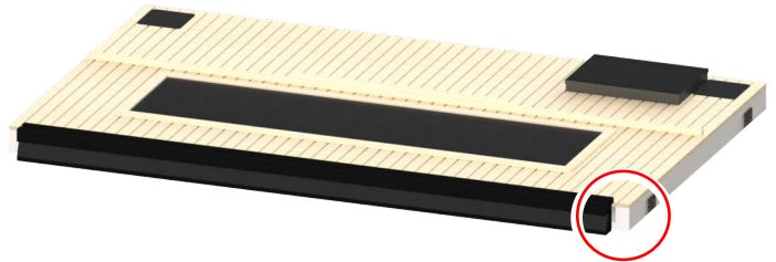
Figure 3. Laying the Floor Panel
