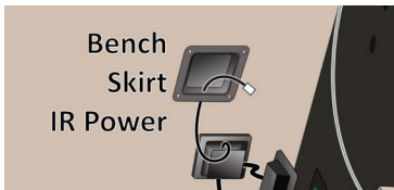
Figure 12. Bench Skirt IR Power Cable
