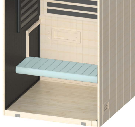
Figure 13. Installing Lower Bench
