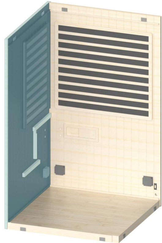
Figure 7. Installing Left Wall Section
