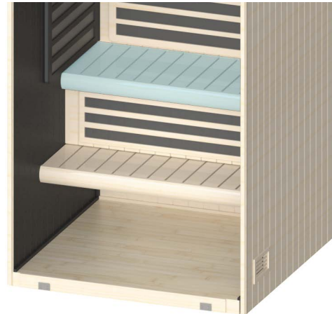
Figure 16. Installing Upper Bench Seat
