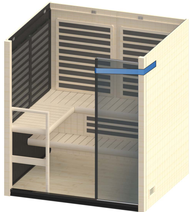
Figure 17. Installing the Single Glass Pane
