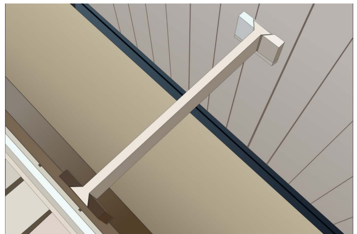
Figure 13. Installing Skirt Support Brace
