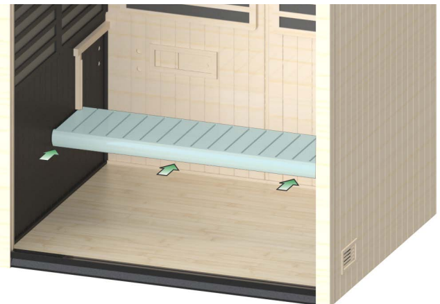
Figure 11. Installing Lower Bench
