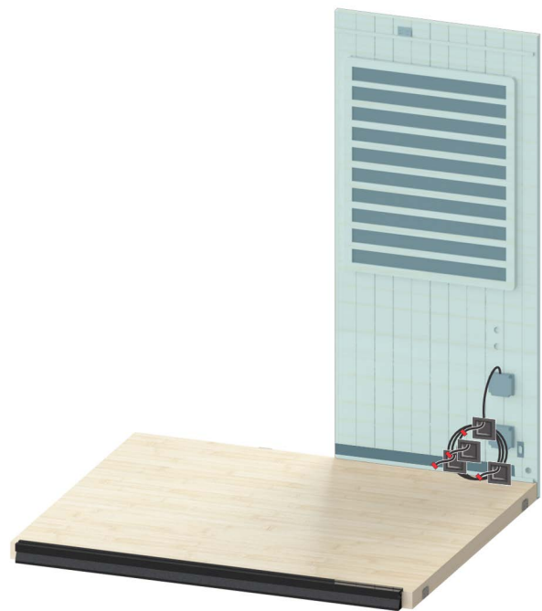
Figure 3. Installing Back Right Wall Section
