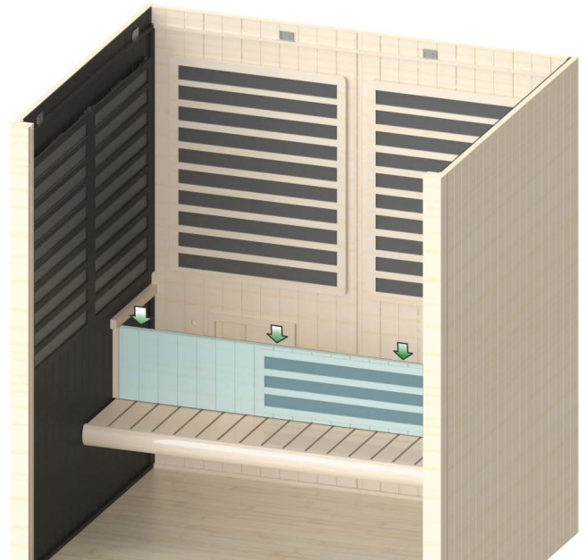
Figure 12. Installing Bench Skirt
