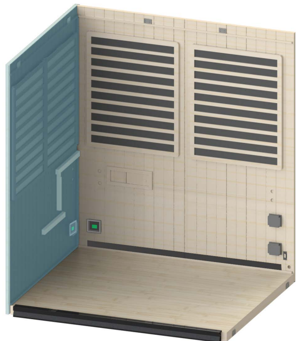
Figure 5. Installing Left Wall Section
