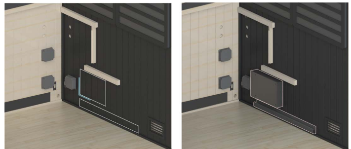
Figure 7. Mounting the CB Box to the Wall
