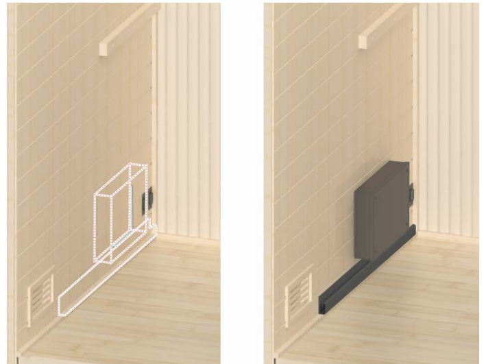
Figure 8. Mounting the CB Box to the Wall
