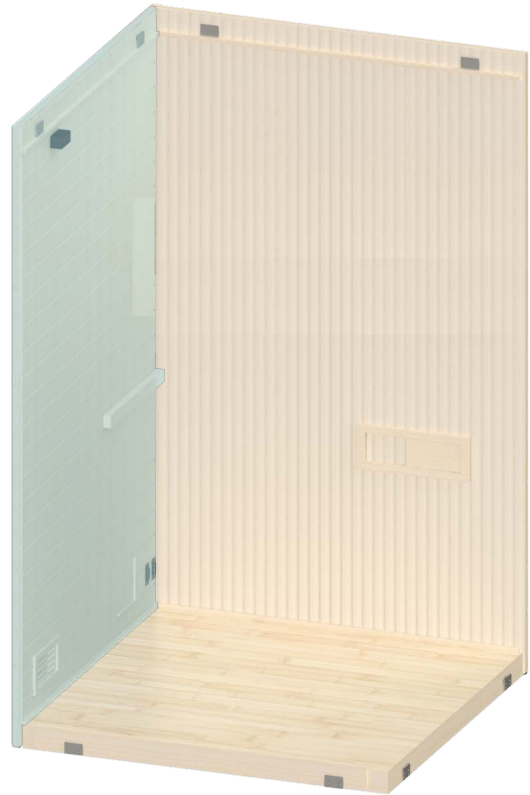
Figure 5. Installing Left Wall Section
