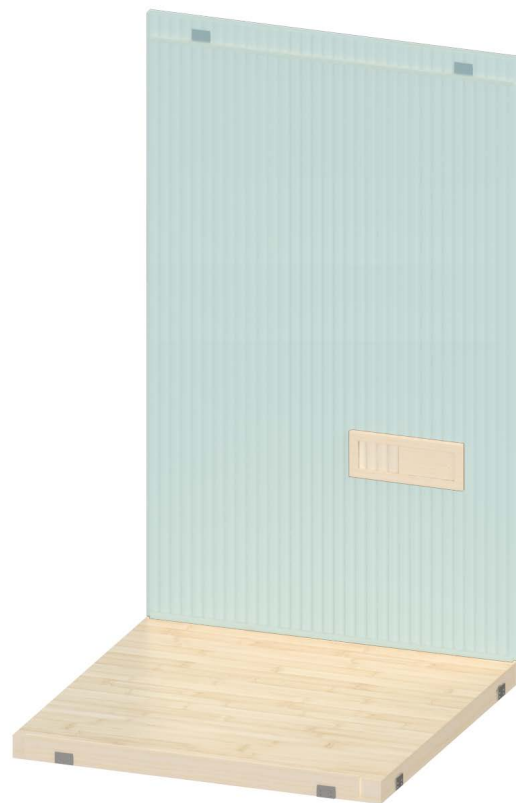
Figure 4. Installing Back Wall Section
