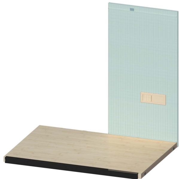
Figure 3. Installing Back Right Wall Section
