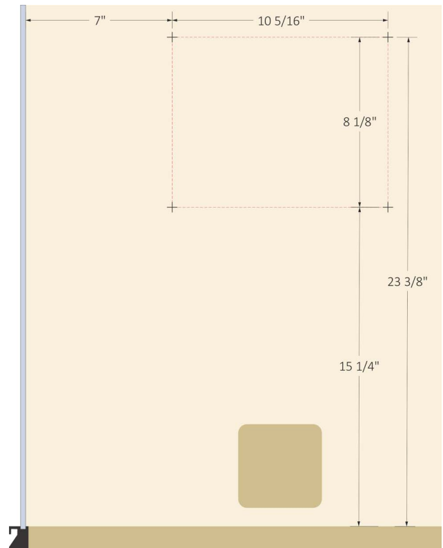
Figure 28. Heater Mounting Measurements
