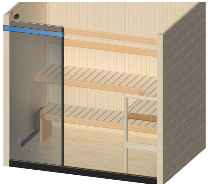
Figure 16. Installing the Single Glass Pane
