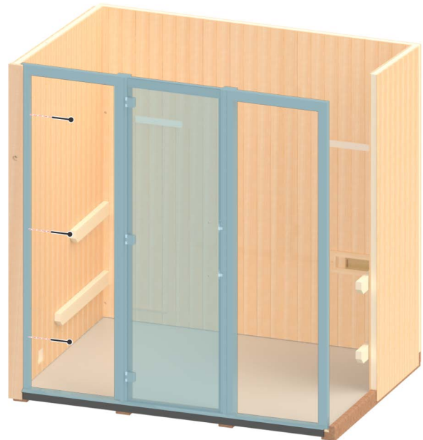
Figure 11. Installing Front Wall Frame Assembly
