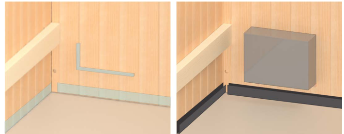
Figure 14. Installing Cable Track and CB Box
