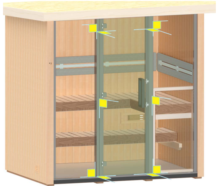
Figure 20. Aligning front wall frame Assembly
