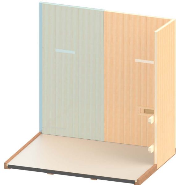
Figure 8. Installing Back-Left Wall Section
