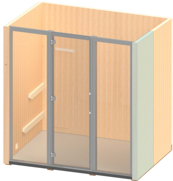
Figure 12. Installing Right-Front Wall Section
