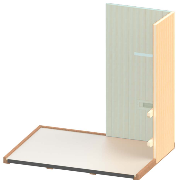
Figure 5. Installing #3 Wall Section
