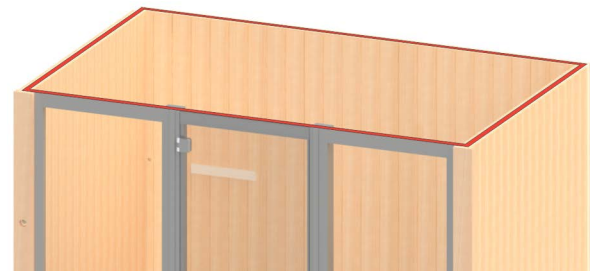
Figure 16. Applying Weather Stripping
