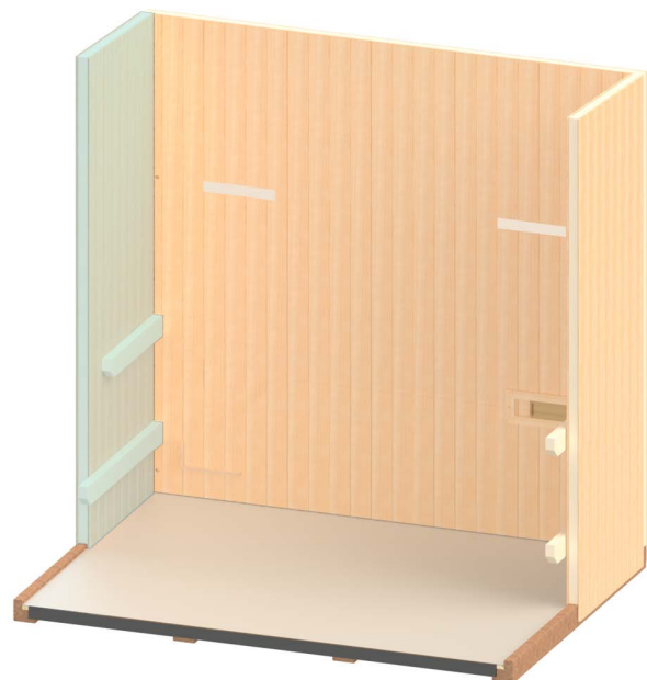
Figure 9. Installing Left-Back Wall Section
