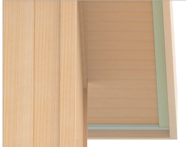
Figure 24. Installing Soffit Trim
