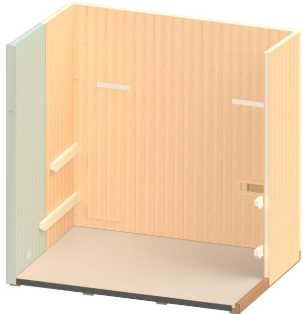
Figure 10. Installing Left-Front Wall Section
