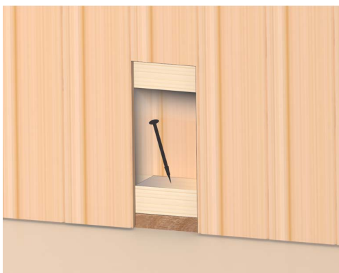
Figure 7. Pockets for Attaching Walls to Base Rail
