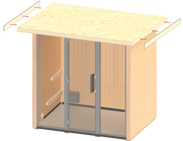
Figure 21. Installing Left and Right Side Wood Fascia
